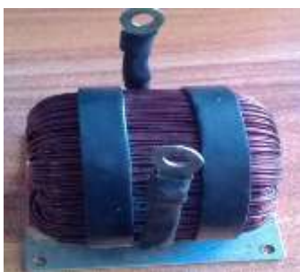
单相滤波电感 F300060*5 150mm*100mm*100mm 150KW 80A 220V
