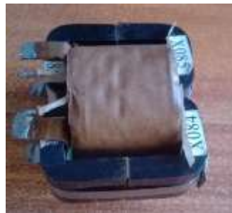
PFC电感 ED16*25*42 62mm*70mm*55mm 5000W 15A 220V
